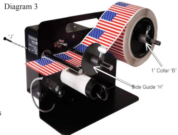
4. Adjust Side-Guide "H" within 1/8" of web, but make sure not to force the web against the side frame of the machine, this will cause tearing.
