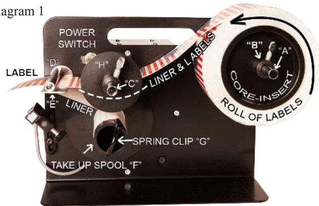
**For rolls with cores smaller than 3":** Follow the directions above, but instead of inserting the core inserts into the roll, just let them rest against the side of the roll instead.
