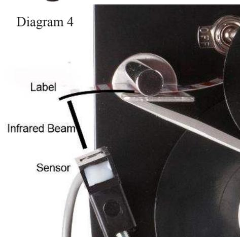
6. **PROBLEM LABELS:** Very thin stock such as acetate, mylar, or vinyl may not release from the carrier paper, but instead will continue down around the table and remain on the carrier. We can provide a special sharp edge plate and tension kit which will usually work for dispensing these labels. (This is already included with the U-25) If you supply us with a sample roll of your labels we can diagnose if the sharp table will work, or what other modification can be made to dispense them.
